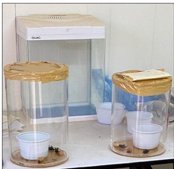
Figure 1. Laboratory assay chamber to evaluate the fumigant action of tested insecticides.
